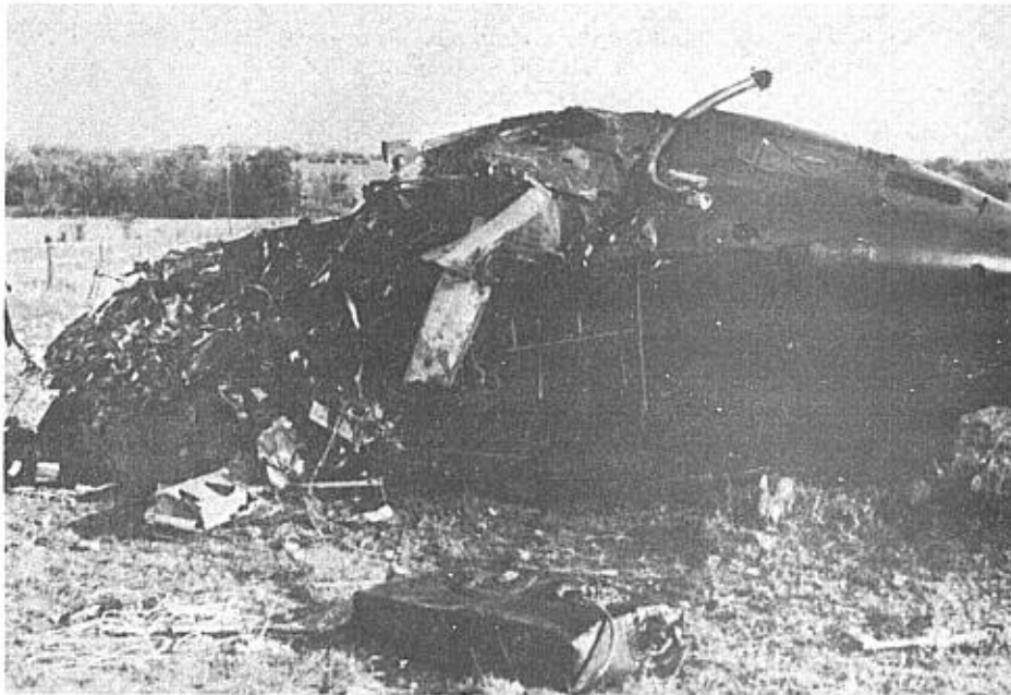
Fig. 2. This UH-1H crashed at night in instrument meteorological conditions (IMC). The pilot and copilot survived with injuries. The crashworthy fuel system functioned as designed. Note the right forward fuel cell in the foreground, which tore loose from the aircraft and prevented fuel spillage. There was no postcrash fire.
